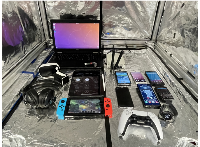
Fig. 5. Interior shot of the Faraday cage we used during our private tests. Our setup and some assorted Bluetooth devices are shown within the cage.
