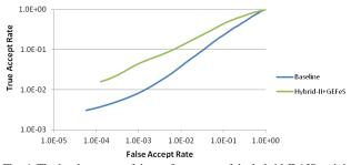
Fig. 6. The log-log curve of the performances of the hybrid-II AIS and the hybrid-II+GEFeS AIS on the English-to-English experiment.
