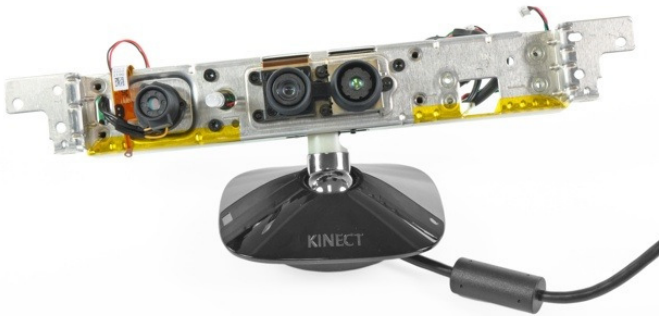
Figure 2: Internals of the Microsoft Kinect [1]
