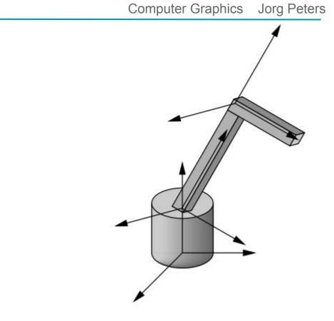
Robot Arm transformations: R (Base) { { T R (lower arm) { T R (upper arm) } }
