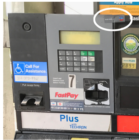
(d) This pump has a single, unbroken seal. It is placed on the hinge of the door, however, making it unlikely to break if the door is opened.
