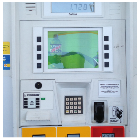
(b) This pump has no seal.
