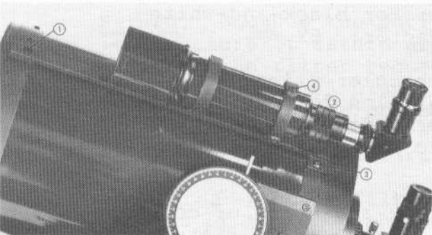
Fig. 13: Using the Erecting Prism. (1) Erecting Prism; (2) Eyepiece-Holder; (3) Eyepiece
