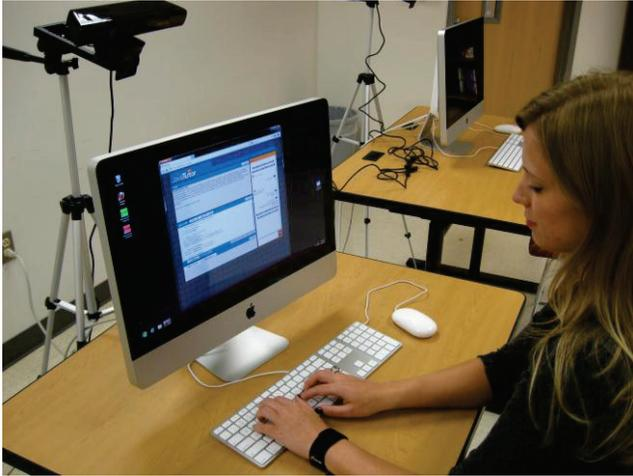
Figure 1. Workstation with Kinect depth sensor, built-in webcam, skin conductance bracelet, and tutoring interface.
