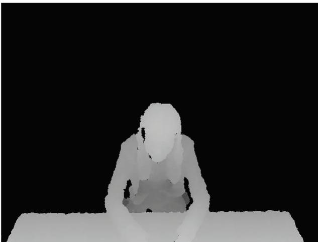
Figure 2. Depth image from the Kinect depth sensor.
