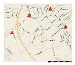
**Fig. 2.** The placement of base stations (red triangles) for a major GSM provider near Virginia Tech. Given that each base station has three sectors, the campus itself receives service from approximately eight total sectors.
